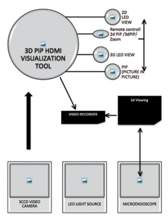
Figure 1: Diagrammatic view of 3d PIP HDMI visualization system and standard 2D Endoscopy system.
